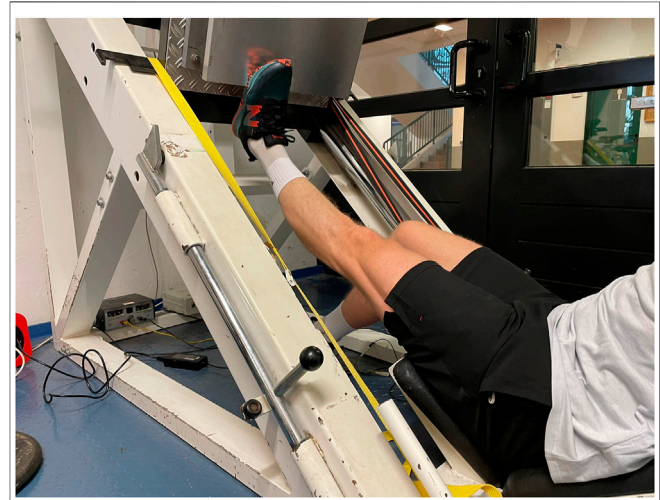
FIGURE 2 | Testing device for maximal isometric strength in extended knee using leg press (LP).
