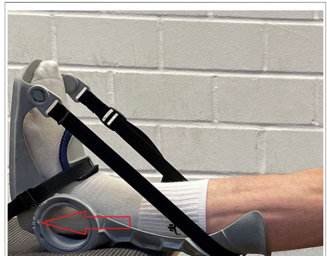
FIGURE 5 | Measuring device for maximal dorsiflexion via goniometer attached to the orthosis.
