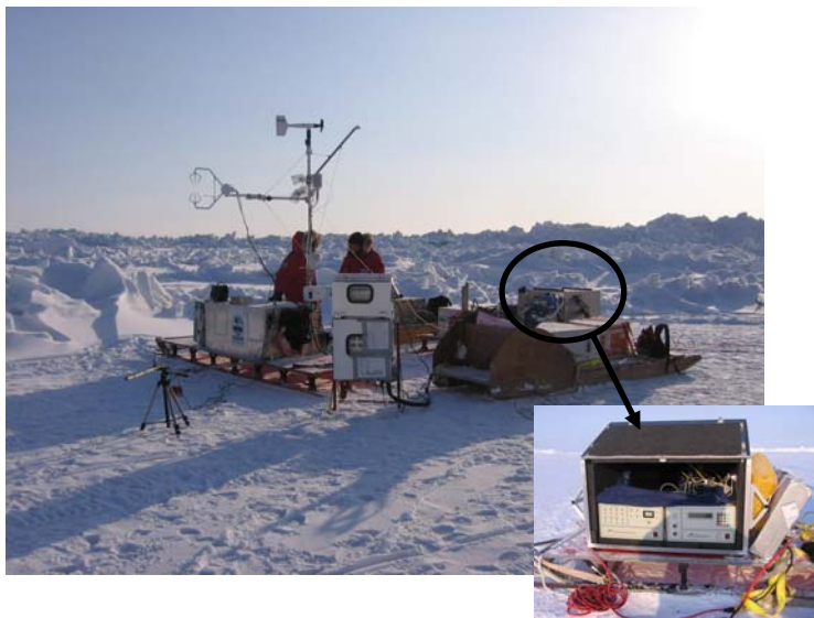
Figure 3b: Atmospheric mercury measurement sample system employed at Barrow, Alaska
