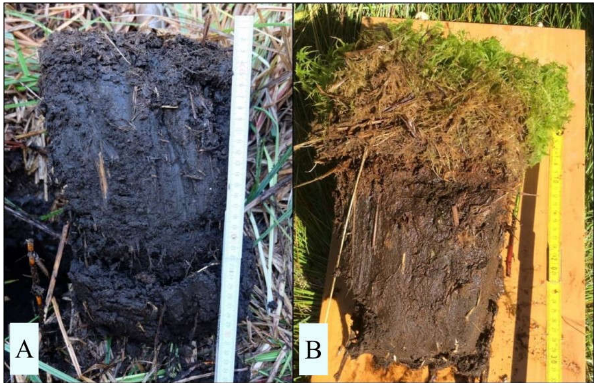
Figure 3.3: Representative peat monoliths of displacement peat and newly formed peat moss peat. A: wet and re-aggregated displacement peat formed by ingrowing and dying sedge roots in the degraded near-surface peat after restoration. B: wet and re-aggregated degraded near-surface peat after restoration with 10 cm of newly formed peat moss peat on top, distinguishable by colour and structure.
