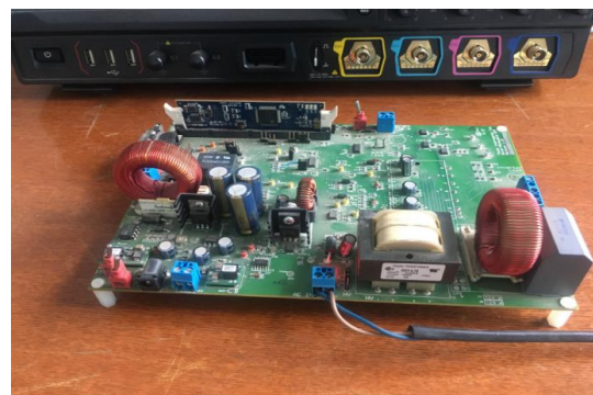
Figure 34. DSP control platform.
