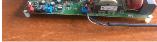
Figure 34. DSP control platform.
