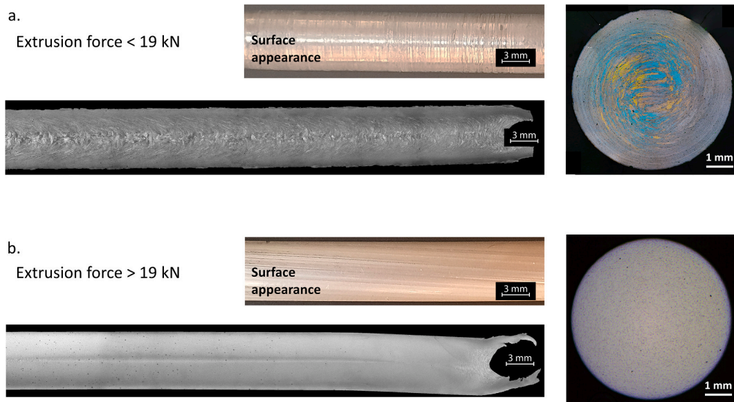
Fig. 3. Macrographs and micrographs of the extruded wires produced by a rotation speed of 300 rpm, extrusion forces lower (a) and higher (b) than 19 kN, i.e. 16 kN and 20 kN, respectively.
