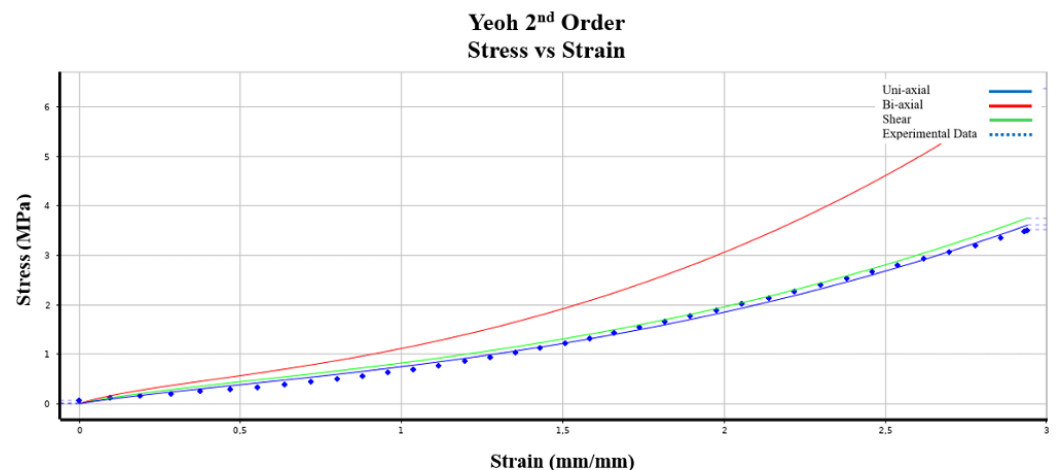
Figure 3. Tensile stress vs. strain responses of five ASTM Type C Mold Max 20 samples.
