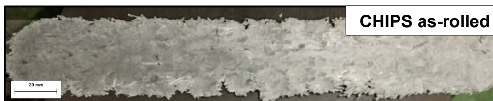
Figure 2. Chips-based as-rolled sheet before ARB process.
