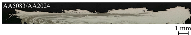
Fig. A.11. Macrograph for FS layer deposited with reversed stud materials, i.e. AA5083 (outer material) and AA2024 (inner material) at 6 kN, 800 rpm and 6 mm/s.
