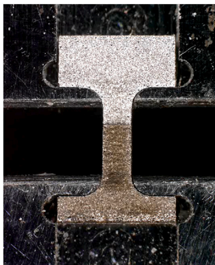
Fig. 3. Micro-tensile test specimen consisting of Al (light) and Ti (dark) inserted in test stage as well as relevant dimensions. All dimensions in mm.
