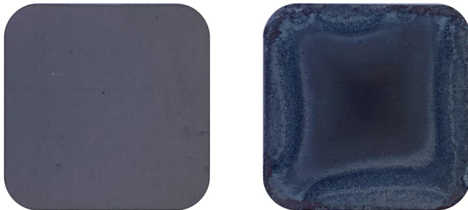
Figure 16. Comparison of specimen contact surfaces pre-sintered in a protective atmosphere (left) and after grinding under argon atmosphere (right), both at 1,100 °C.
