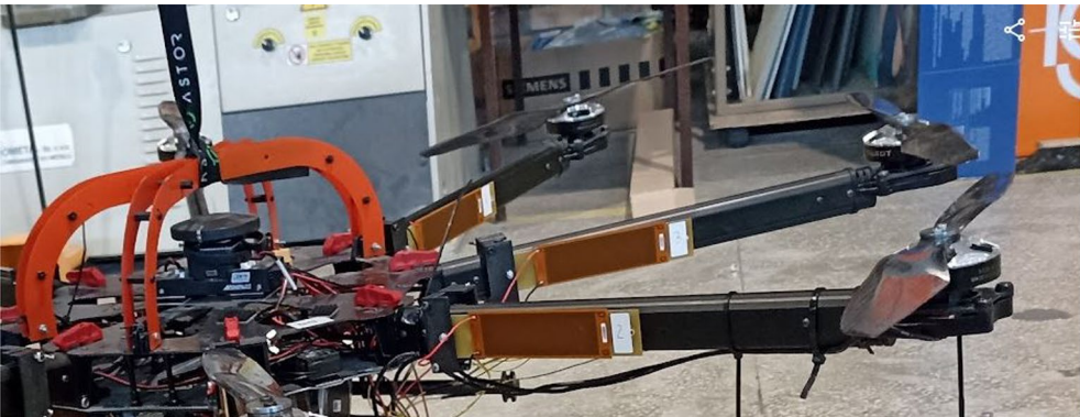
Fig. 3. Illustration of piezo composite sensors located on the side plane of the UAV arm.
