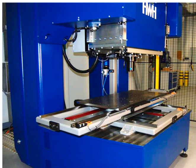
Fig. 2. Harms & Wende® RPS200 machine used to produce welds in this work.
