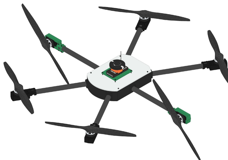
Figure 2. Proposed HTR with two servomotors tilted 90°.
