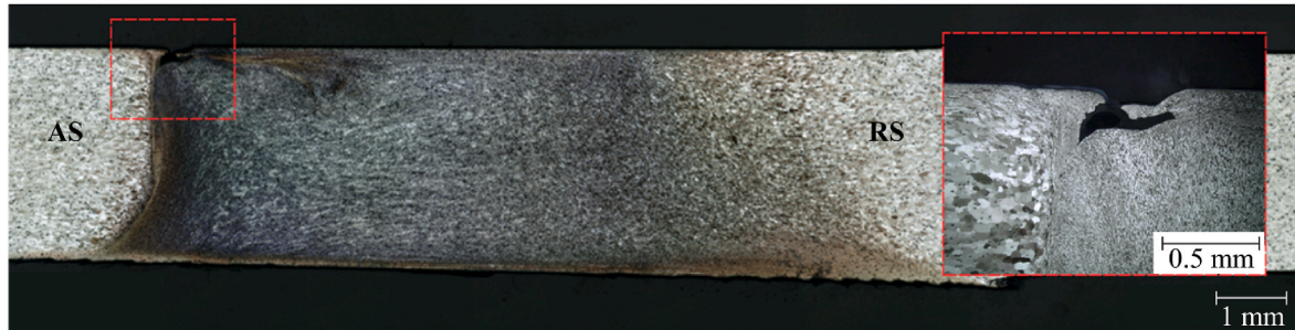
Fig. 4. Macrograph of the SSBT-FSW joint produced at a welding speed of 200 mm/min, showing the presence of a surface defect on the advancing side. Therefore, for SSBT-FSW a lower welding speed of 150 mm/min was chosen in this study.
