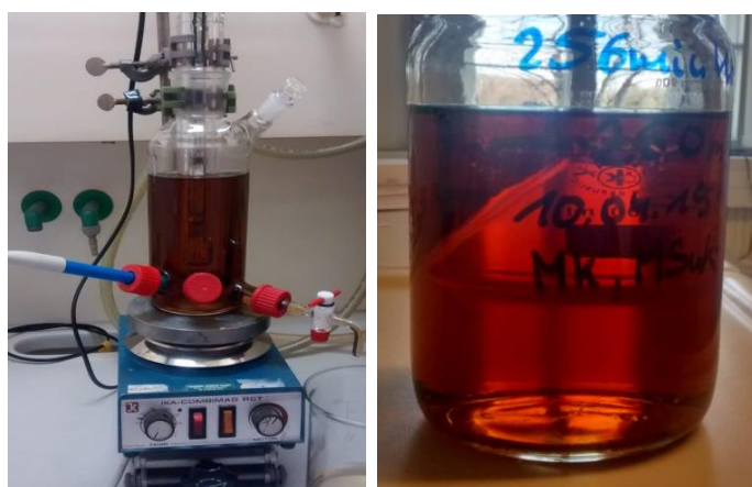
Fig. 8: SPX solution after 128 min (left) and 256 min (right) of photolysis
