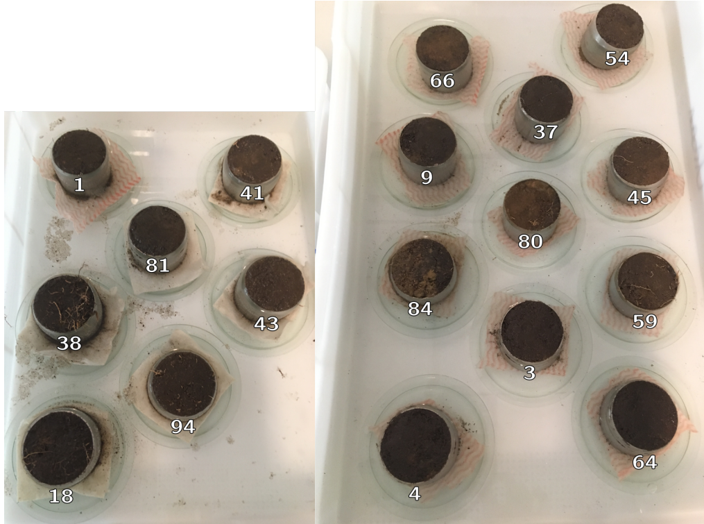
Fig. 11: Volume samples in water basins with added cylinder numbers (see 3.1 & Appendix B, App. Tab. 7)
