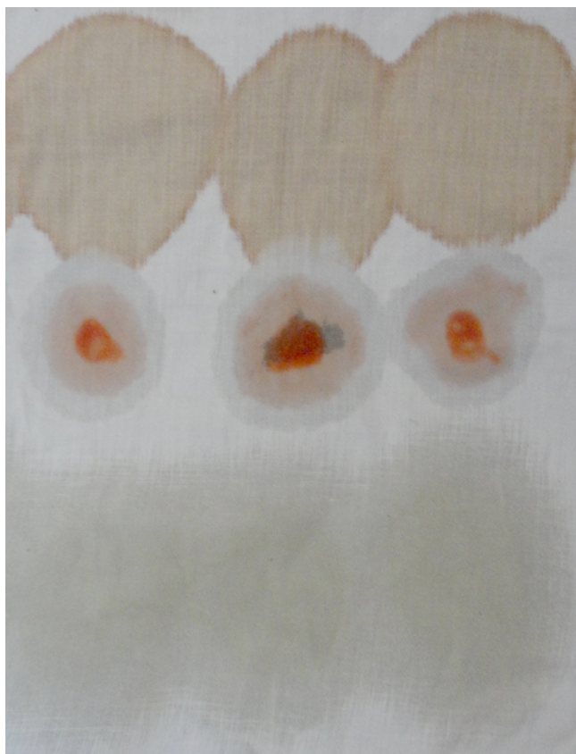
Fig. 4: Replicable stains on undyed cotton satin. From top to bottom: Balsamic vinegar, tomato juice, and rapeseed oil
