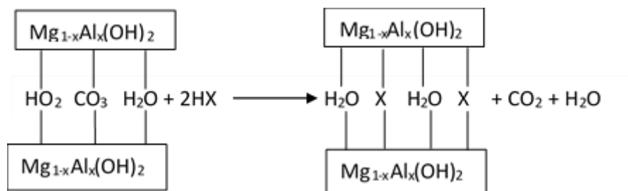
Figure 12 The mechanism of the hydrotalcite compound (Endres et al., 1991)
