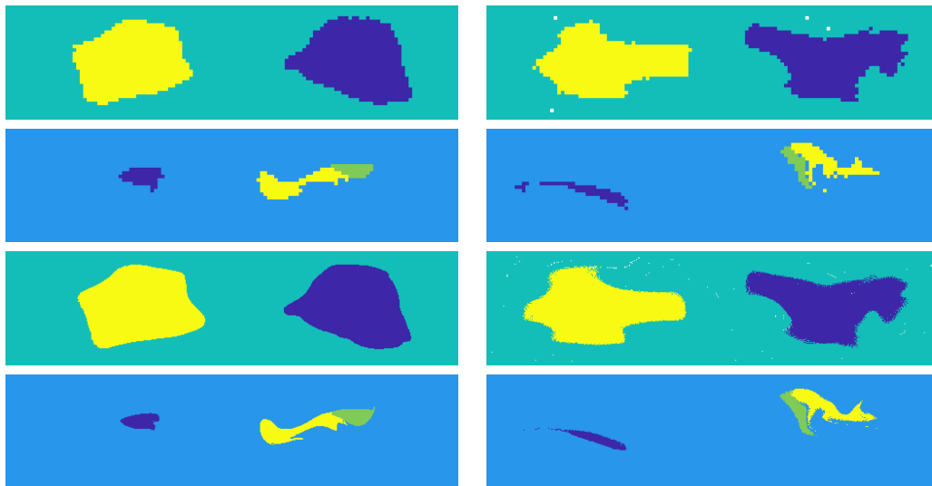
Figure C.6.: Extracted coherent sets at initial time (left column) and final time (right column) via an application of the standard k -means algorithm. The first two rows show these for the short time interval and long time interval using 2^{12} boxes. The last two rows show these using 2^{16} boxes and 16 test points per box.
