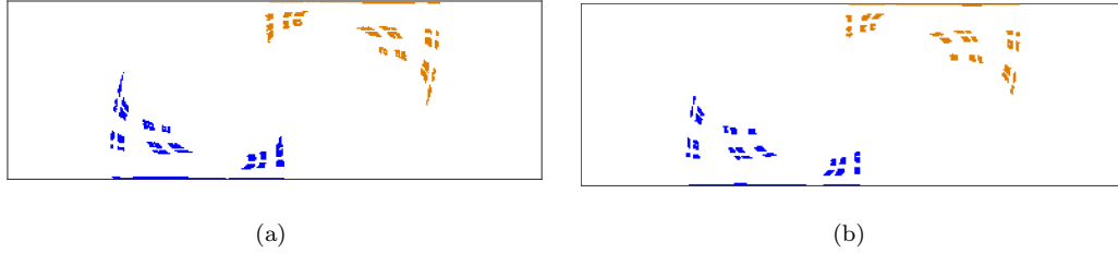
Figure 7.5.: Self-communicating classes of P for the double gyre mixer with system parameters \alpha = 0.5 , \epsilon = 0.4 , and \beta = 0.5 (a) and with system parameters \alpha = 0.5 , \epsilon = 0.35 , and \beta = 0.5 (b). There are two self-communicating classes: Boxes that belong to the first self-communicating class are colored in blue and boxes that belong to the second second are colored in orange.
