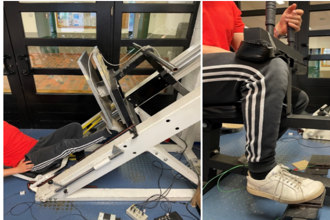
Figure 7: Maximum strength testing for the plantar flexors with extended knee joint (a) and with flexed knee joint (b)
