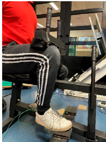
Figure 1. Calf-muscle-testing device (CMD) measuring the maximum isometric strength in pre- and post-test with force plates.
