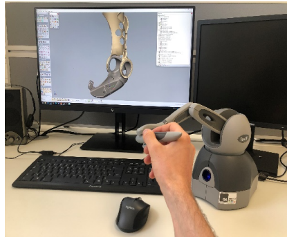
Figure 5: Designing a professional stretching orthosis using Geomagic Free Form
