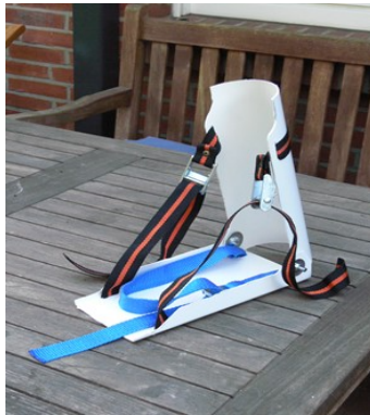
Figure 4: Second self-conducted orthosis to check different types of material and the possibility of mass production
