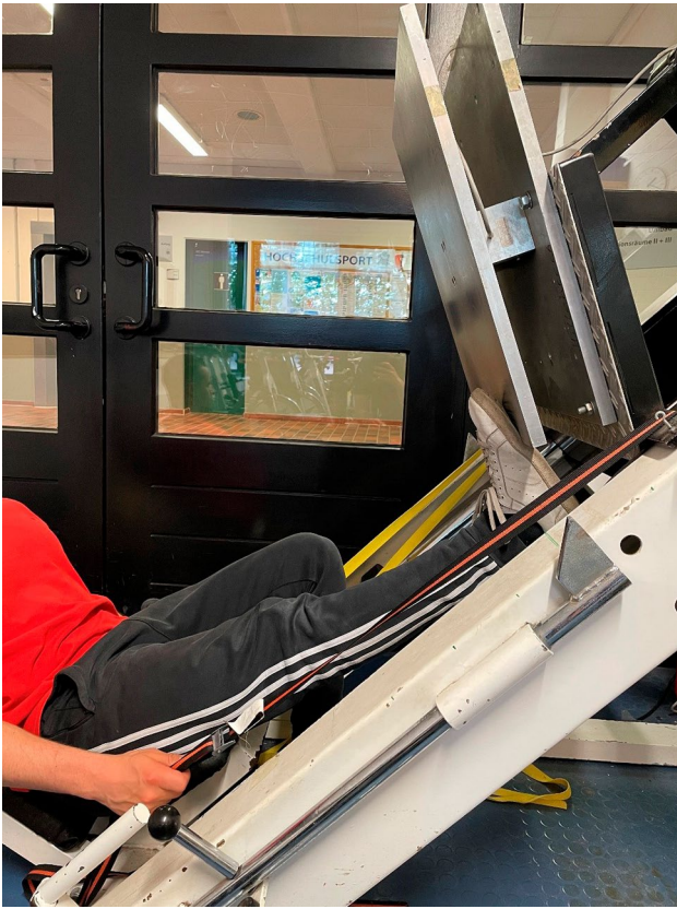
Fig. 2 Leg press testing device for maximal isometric strength with extended knee joint (MVC180)
