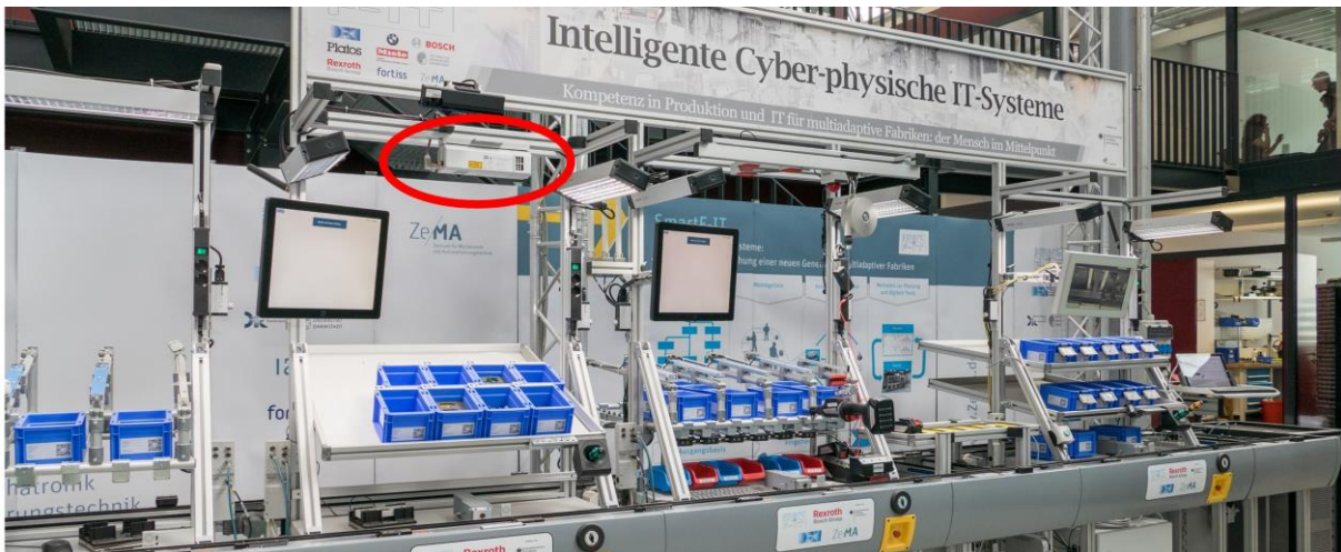
Figure 39: Laser system integrated into an assembly line (with courtesy of ZeMA gGmbH)
