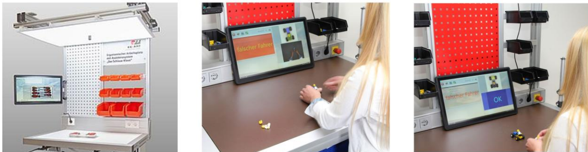
Figure 25: Assembly and quality inspection system (RK Rose+Krieger GmbH, 2022)
