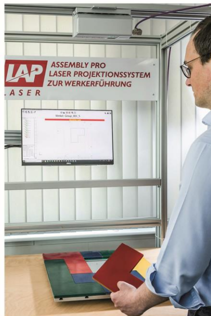
Assembly station with laser projector
