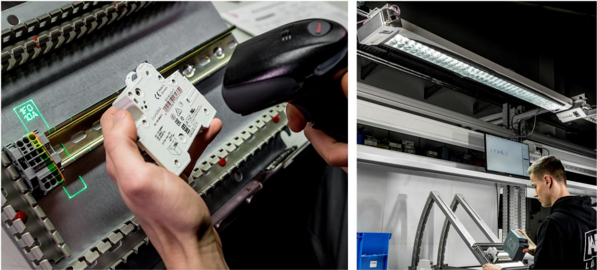
Figure 38: Electrical cabinet assembly (with courtesy of LAP GmbH Laser Applikationen)
