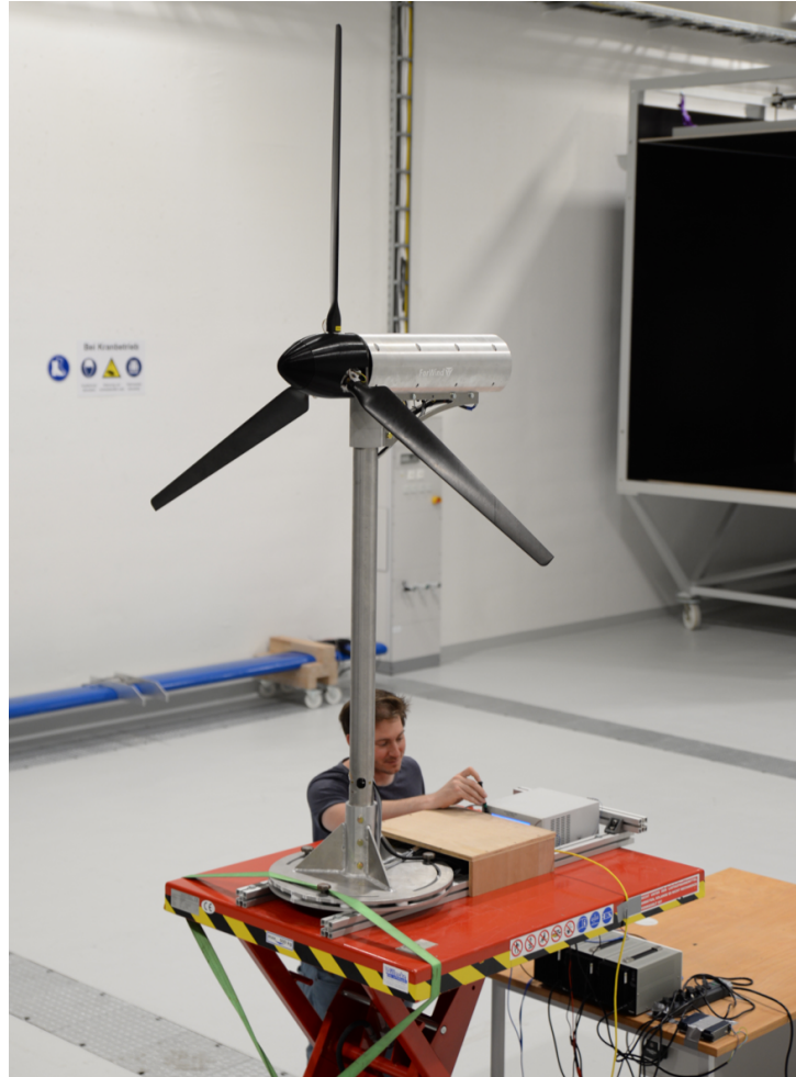
Figure 4.1: Model Wind Turbine Oldenburg (MoWiTO) with a rotor diameter of 1.8 m operated in the WindLab at ForWind Oldenburg.
