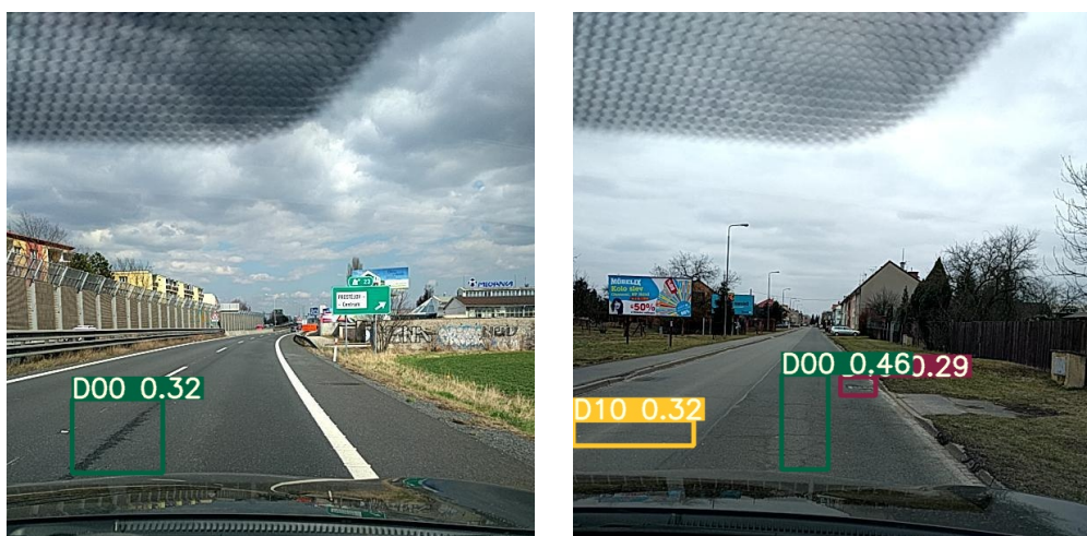
(a) Repaired crack misclassified as long. (b) Manhole cover misclassified as a pothole (D40, red) (D00, green)
