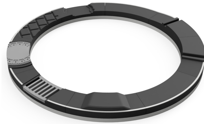
Figure V.6: The nine mounted road elements on the slewing ring
