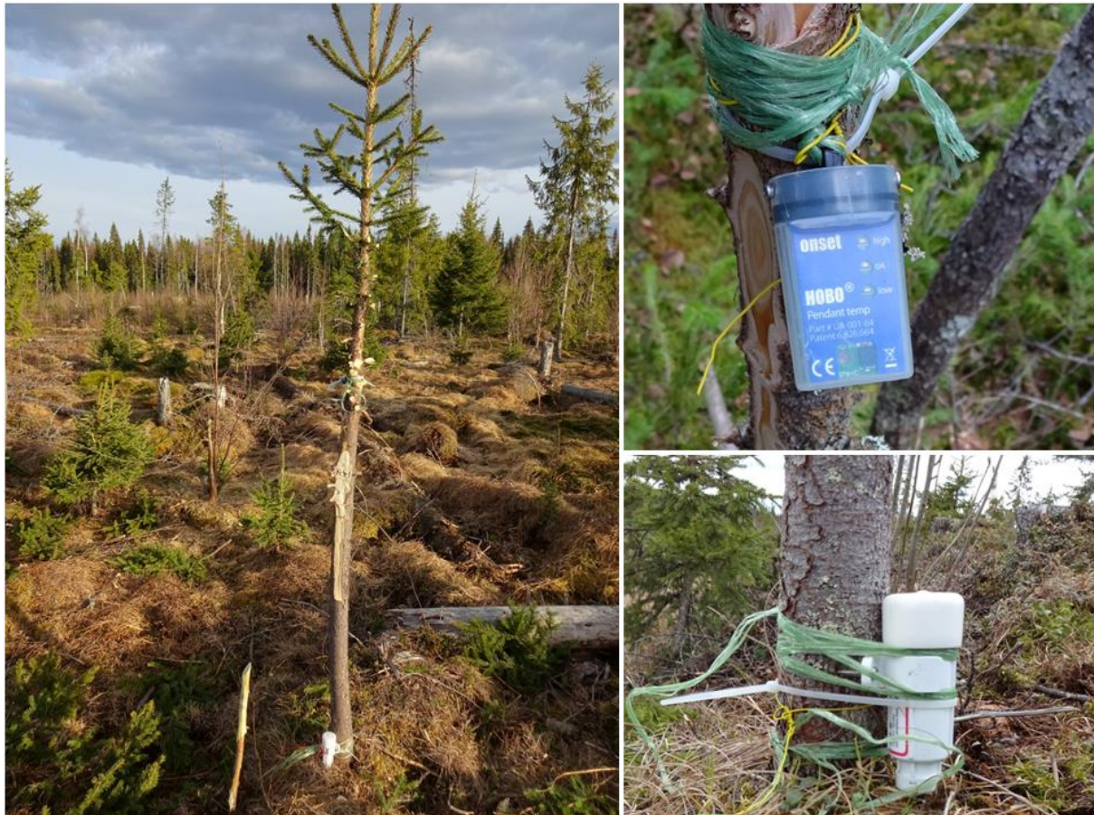
Figure 3: Microclimatic data-loggers installed at a small tree in the centre of a study plot. Top: Data-logger measuring temperature at 1.3 m. Bottom: Data-logger measuring temperature and relative humidity at ground-level. Pictures were taken by JSB.
