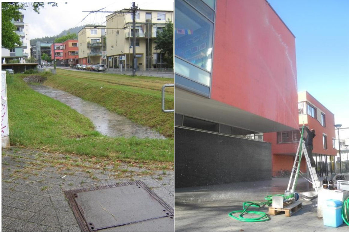
Figure 2: Left: Swale S1 after a storm event (Sub-catchment 1 with arcade-like overhanging facades in the back; red facade = facade of sprinkling experiment). Right: Façade during sprinkling experiment (since façade overhangs a paved surface, façade wash-off is connected to the storm drainage and the capturing BR facility)
