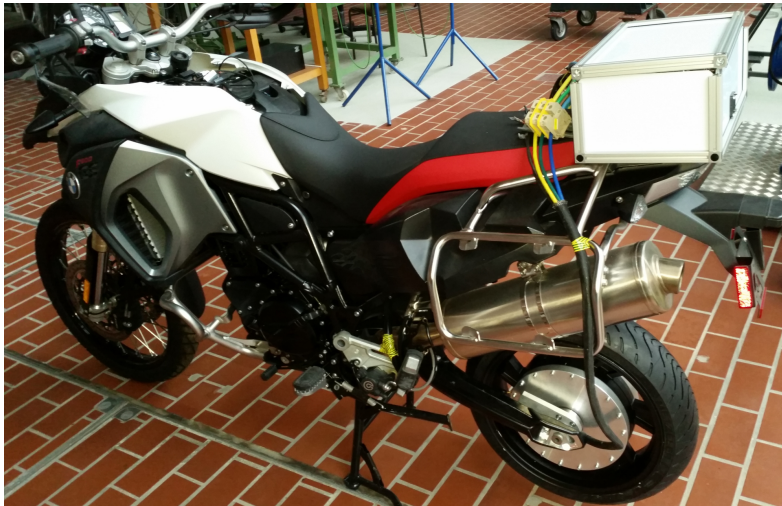
Figure 7.1: Hybrid motorcycle (work in progress), based on a BMW F 800 GS Adventure with a PMSM.
