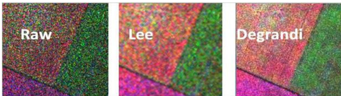
Figure 9: Effect of using Lee and De Grandi filters on removing the speckle noises.
