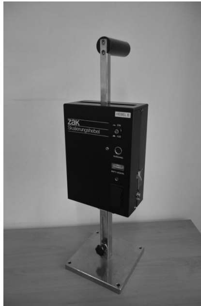
Figure 12. The adapted model of the Vehrs lever used in this study.
