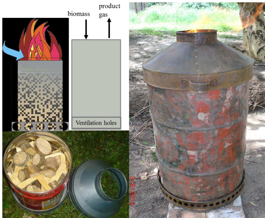
Figure 2.6: Illustrated functions of biochar kiln (left), and biochar kiln used for producing biochar to apply in present research (right)
