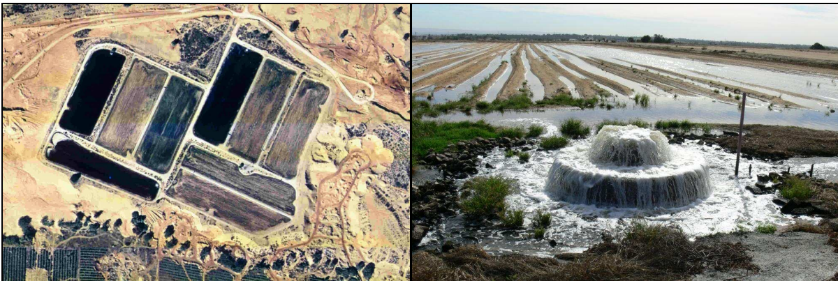
Figure 1-3 Aerial view of several percolation basin within the Shafdan SAT site in different states of flooding (left, picture kindly provided by Prof. Lev, Hebrew University, Jerusalem, Israel) and flooding of a percolation basin with treated wastewater after ploughing (right, picture taken by the author).
