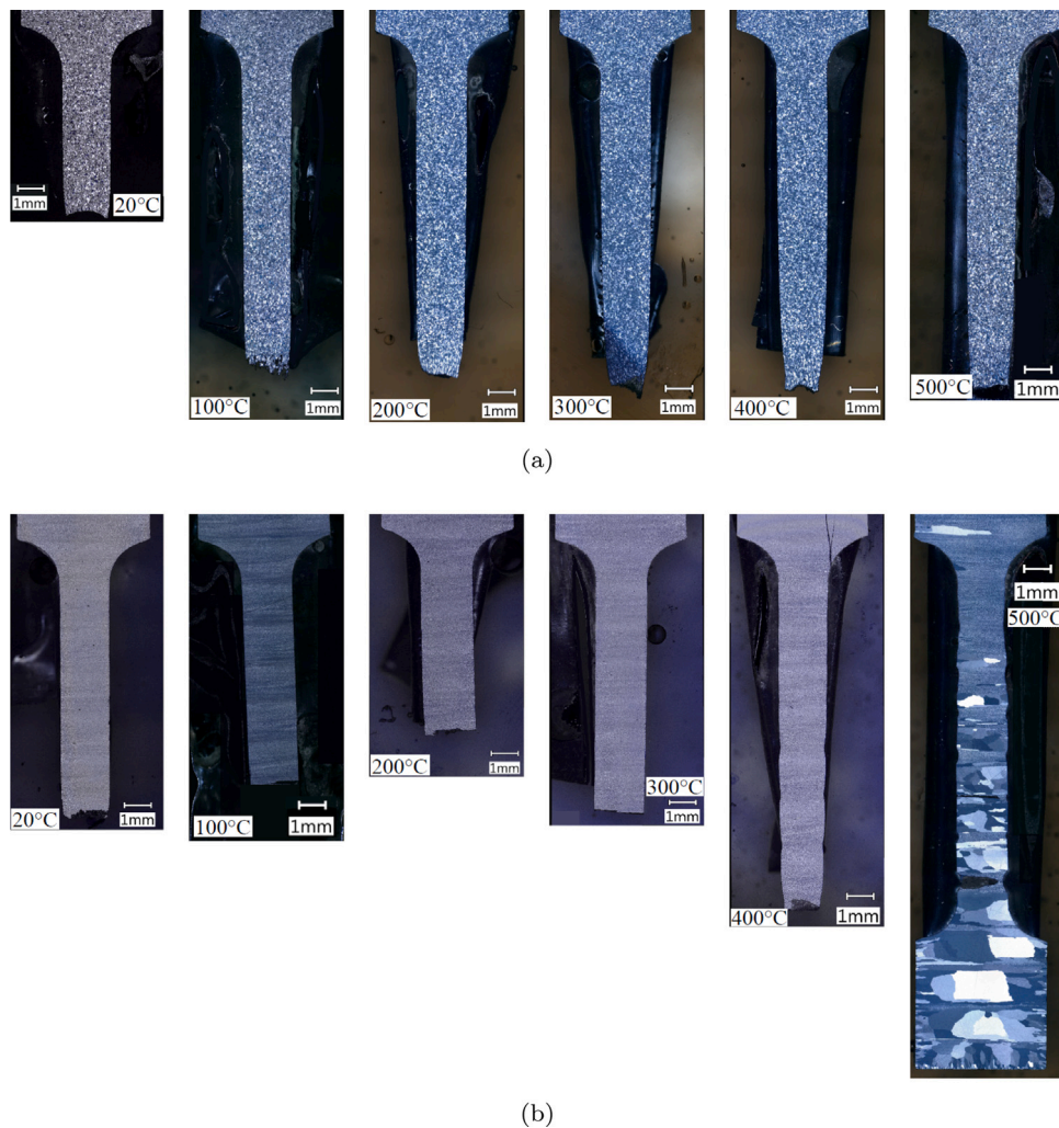
Fig. 5. Exemplary polished and etched MFTT specimens from BM (a) and MLFS material (b) tested between 20 °C and 500 °C.
